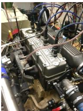
G432 engine (4 cylinders, \phi 102/120\text{mm} , VTG) in CTU lab
