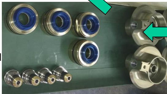
e) Damper parts manufacturing and assembly
