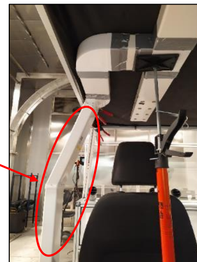
Realization of Ceiling-based displacement ventilation system in cabin mock-up
