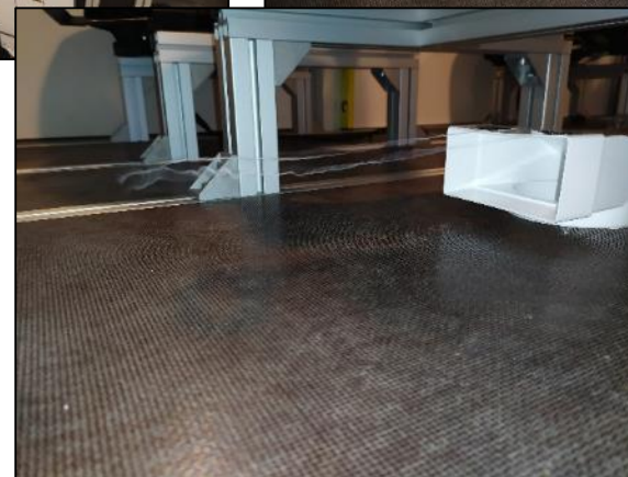
Realization of Local air distribution under seats
