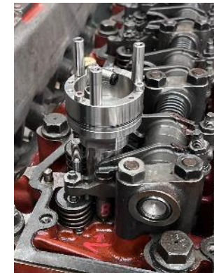
3-WP07-004 - 005 Active pre-chamber optimized for multi-fuel operation
