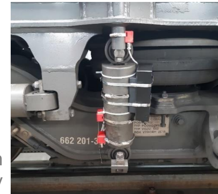
Experimental measurement unit on vertical secondary damper of 10Ev
